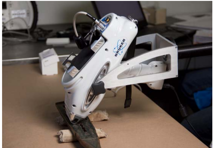
Further elemental analysis was performed using non-destructive X-ray Fluorescence Spectroscopy (pictured) and also with Scanning Electron Microscopy to help determine what pigments were used in the paint.
